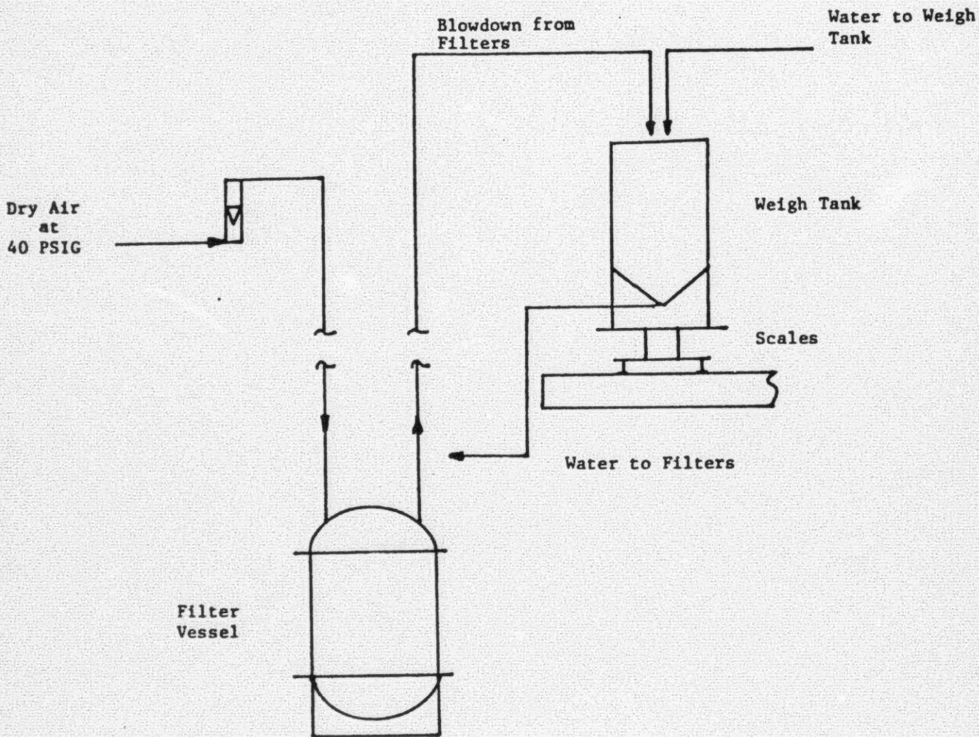
BLOWDOWN SETUP FOR CNSI-TMI FILTERS
