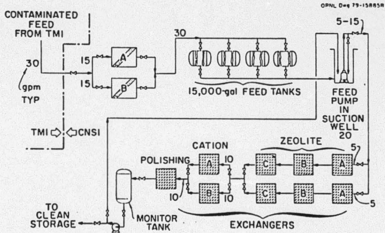
Fig. 12. Liquid waste decontamination flowsheet.
